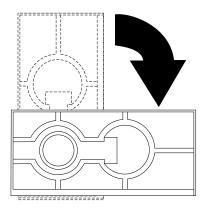
When you are finished installing options and have installed the side cover, turn the two front stabilizing feet a quarter turn out from the server and set it carefully back on its feet.
